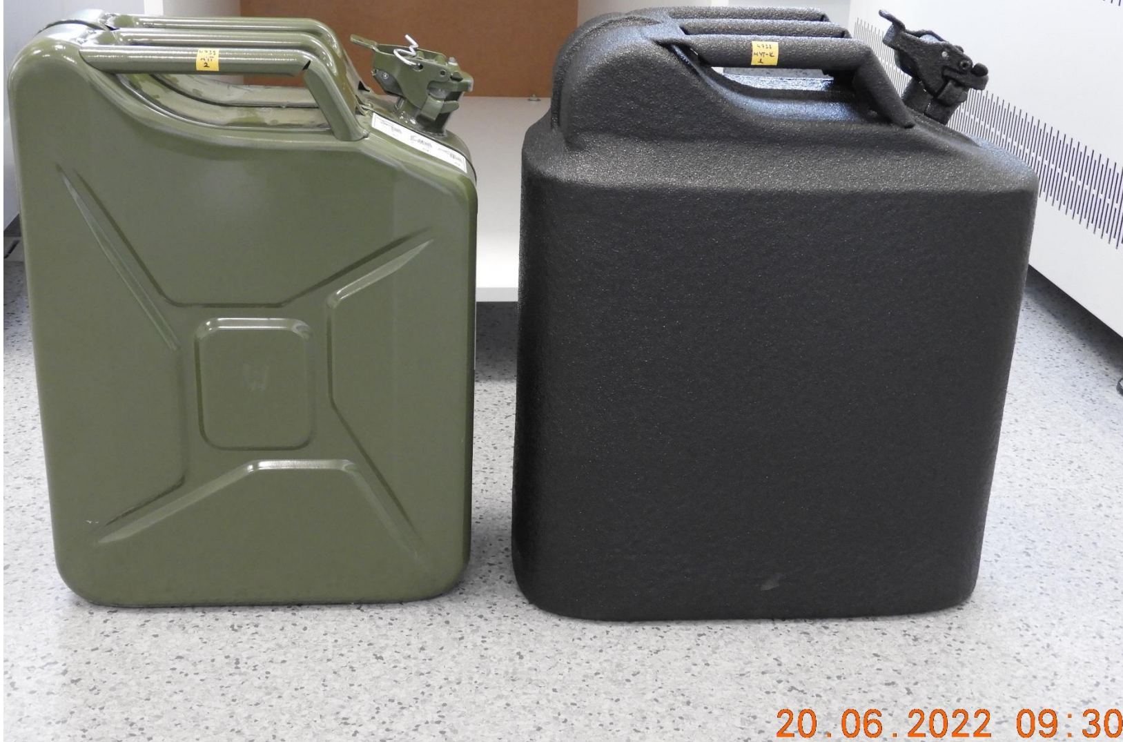
Low Temperature Test, MIL STD 810G Method 502.5, Procedure I (4 hours at -32 °C) Before the Test
